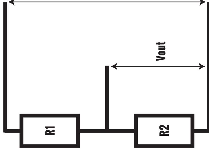
See the diagram on the left for a representation of a potential divider. Calculate the value of the output voltage from a potential divider with the formula:
